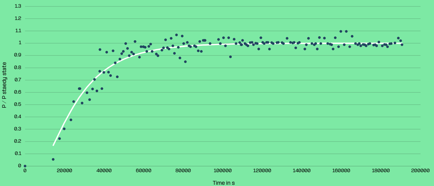
Figure 5 Example of an experimental non-steady state hydrogen permeation result at room temperature and hydrogen pressure =700 bar as measured on 2mm thick plaque.
