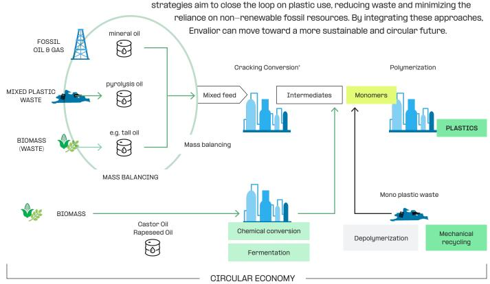
\* Chemical recycling denotes mainly the conversion of mixed plastic waste via Pyrolysis – this pyrolysis oil is then fed into the cracker system.
