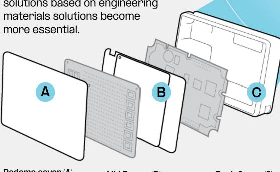
Radome cover (A) good performance requires low dielectric losses Mid Frame (B) good performance requires very low radar reflecting materials
