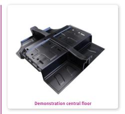
A vehicle central-floor module from carbon fiber-reinforced PA410 made by FCA (EU-sponsored ENLIGHT project). The UD tapes based ply-books were thermoformed to the final shape. The composite part is 18% lighter than state-of-the-art, steel-based designs, while still fulfilling safety requirements. The composite strength and dimensional stability are not affected by the E-coating process, a requirement of BIW parts.
