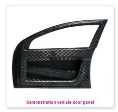
A demonstration vehicle door panel made by JLR from carbon fiber-reinforced PA410, as well as fabric sheets woven from the same UD tape (EU-sponsored ENLIGHT project). The UD tape products were thermo-formed and glued to make the panel, which is 60% lighter than state-of-the-art, steel-based designs, while still fulfilling safety requirements. The full composite door consists of structural panels and a tape-wound side impact beam over an extruded, permanent mandrel.
