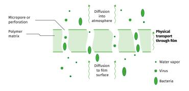
High to very high MVTR materials, with tunable O2 permeation and water absorption characteristics
