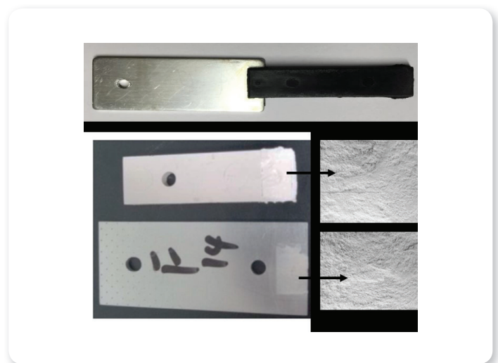
Figure 6: Above is a shear specimen produced with NMT to join the polymer to the metal substrate. Below is a specimen after testing showing that performance was not limited by the interface leading to excellent bond strength.
