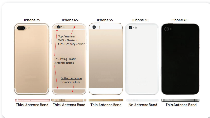
Figure 2: Different generations of iPhones showing the evolution of antenna separators (Source: manually cut and paste from various internet pictures, logos manually deleted)
