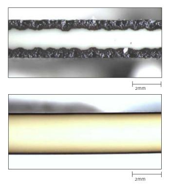
Figure 4 — Parts based on materials with (R) and without (L) the Diablo solution after aging at high temperatures
