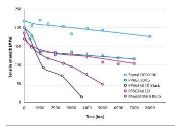
Figure 5 — Tensile strength retention of Stanyl Diablo versus other materials
