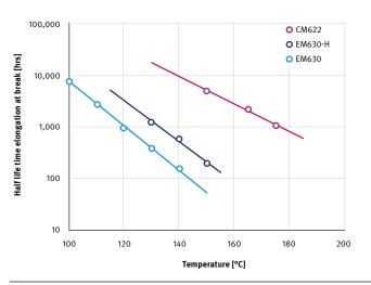
Figure 3 — Comparing the effect of adding a stabilizer and improving the intrinsic stability of the polymer backbone on retention of properties
