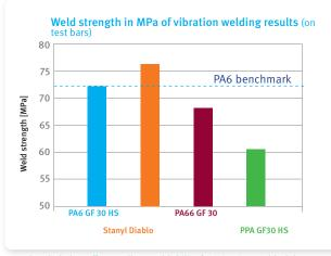
Stanyl and Akulon offer excellent weldability for injection molded ducts.
