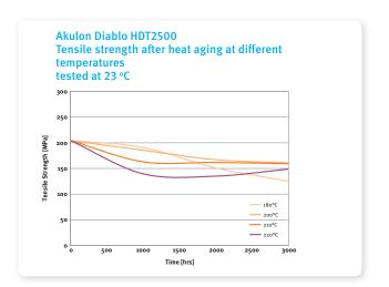
Akulon Diablo fills the gap between Akulon PA6 and Stanyl Diablo by combining long term heat aging performance and mechanical properties at 180-200°C.
