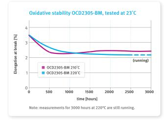
The material's elongation at break remains stable above 2%, even after 3000 hours of heat aging (measured on tensile bars).
