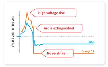
Fig.4 Arc quenching performance
