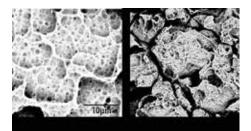
Fig. 2. Scanning electron microscope images of substrate structures made of aluminum (left) and stainless steel (right) that are suitable for an NMT connection (© DSM)
