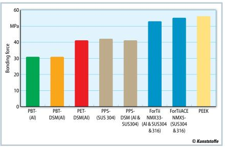
**Fig. 4.** In a comparison of the bonding strength of various plastics on stainless steel after NMT processing, the new materials stand out with high values (AI = aluminum, SUS 304 and SUS 316 = steel alloys) (source: DSM)
