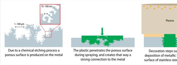
Decoration steps such as PVD deposition of metallic layers on the surface of stainless steel or titanium
