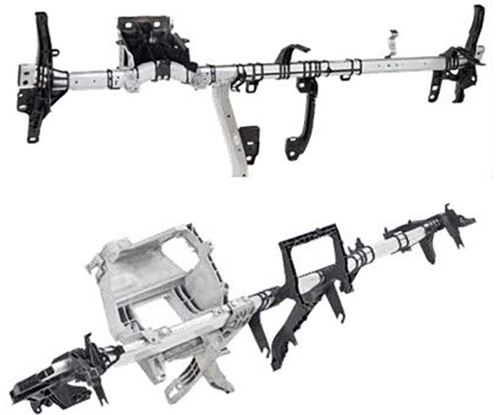
Examples of cross-car beams created using hydroforming hybrid process.
